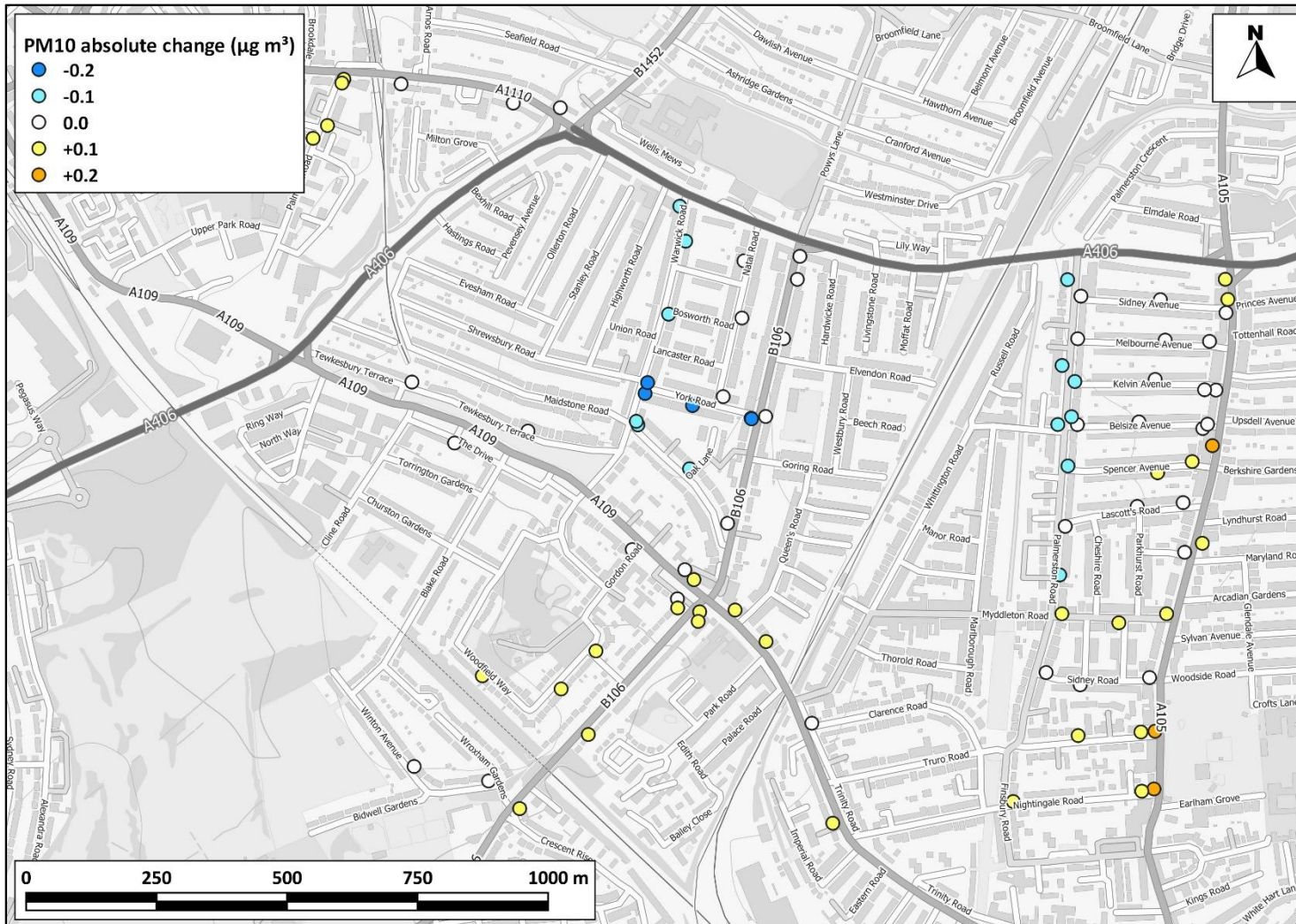
Figure 10: Predicted Changes in Annual Mean PM 10 Concentrations with Quieter Neighbourhood Scheme in 2020(µg/m 3 )
